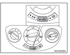
Press this button when driving in dusty conditions or to avoid traffic or outside fumes, and when quick cooling or heating of the passenger area is required. The indicator light will illuminate and interior air will be reclaculated.
